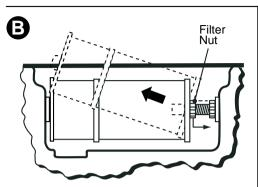
Loosen filter nut to provide clearance, then remove filter assembly.
