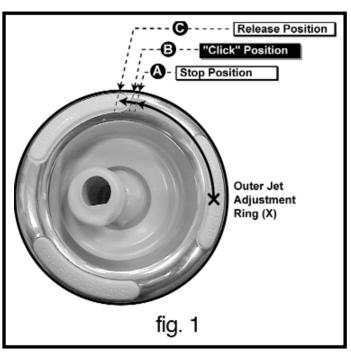
internal between positions (A-B), however, additional force is necessary at position (A) to unlatch its retaining mechanism from the wall fitting.
