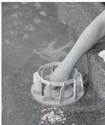
2) Screw filter cartridge in place
