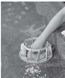
Turn filter cartridge counterclockwise to unscrew.
