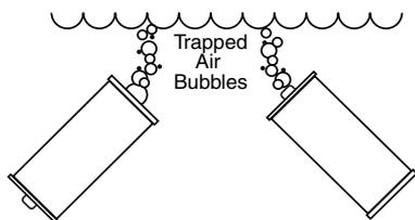
Submerge new filter cartridge in spa and tilt each end upward to remove most of the air bubbles trapped inside the filter.
