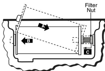
1. Install new filter cartridge, then tighten filter nut until it just touches filter face. **DO NOT OVERTIGHTEN!**
