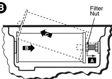
Loosen filter nut (A) to provide clearance, then remove used MicroClean II filter cartridge (steps B-C).
