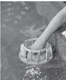
Turn filter cartridge counterclockwise to unscrew.
