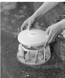
3) Snap Vortex filter top in place
