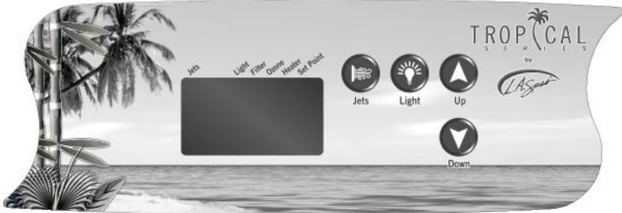
Single Pump K-71 Tropical (Kona) Control System
