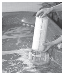
1) Center filter cartridge over canister
