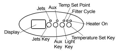
Default System Operation: When power is applied, or there is a temporary loss of power, the system will initiate its default programming. The filter cycle will begin24-hours after the system has been powered up. The filtration cycle will be active for 1-hour and will repeat every 12-hours. The temperature will be maintained at 95° F. NOTE: Default Setting can be changed without notice.
