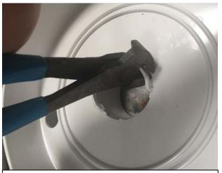
With end-cutting pliers, cut off the tabs, as close as possible to the base.
