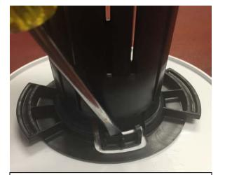
Remove the EZ-lock filter screen by inserting the screwdriver in the clip, pry it towards the outside and lift on that side. Once loose, jiggle the EZ-lock towards the opposite side and lift.
