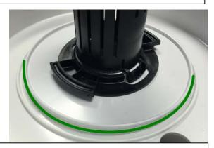
Align and mount the repair plate on to the filter bottom. Hold in place for about a minute. Finish by adding a large bead all around the plate to for better seal.
