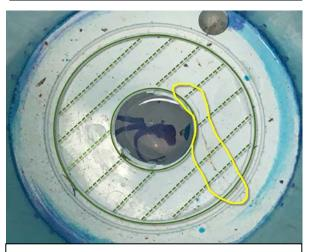
Apply a coat of epoxy to completely cover the crack (yellow area) followed by a bead over the green line circle and dotted lines.
