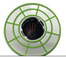
Apply a bead of epoxy all over the green lines as shown. Act fast to prevent the epoxy from drying/curing.
