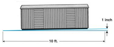
Slope 1 inch per 10 ft. for proper drainage.
