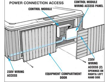
IMPORTANT: The following must be followed to properly install the equipment compartment door or wiring access panel.
