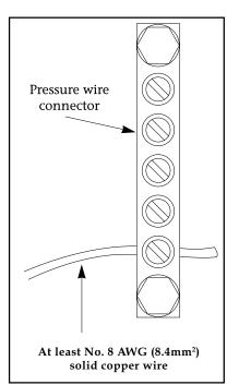
Located on the side of the spa pack box for M Class Equipment Systems and on the heater for S Class Equipment Systems
