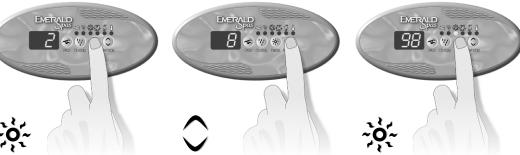
Press and hold Light key for 5 seconds. The display will show a value that represents the filter cycle duration in hours. Use Up/ Down arrow key to change setting.
