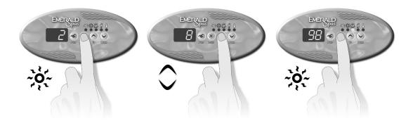
Press and hold Light key for 5 seconds. The display will show a value that represents the filter cycle duration in hours.
