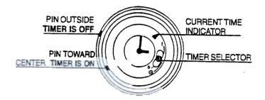
The timer which is located on the front panel of the control box, controls the low speed pump only. All other functions of the spa are accessible regardless of the timer setting.
