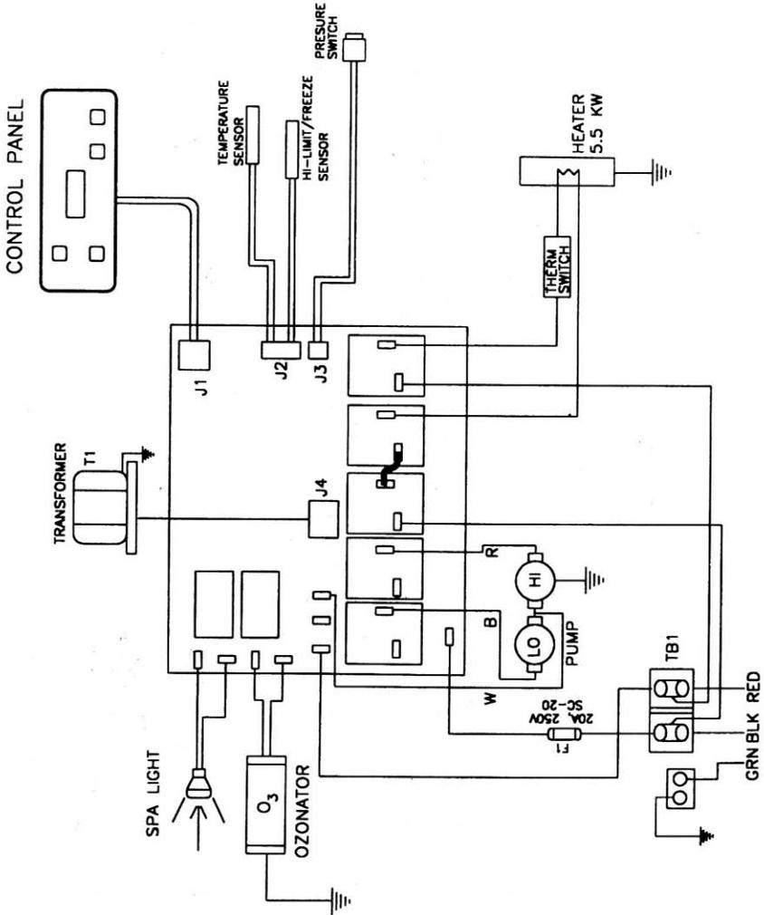
240 VAC, 1 PHASE, 50/60 Hz USE COPPER CONDUCTORS ONLY Wire size must be appropriate per NEC and/or LOCAL CODES.
