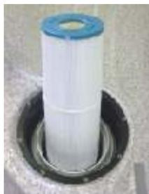
Pull tab and turn lock ring counterclockwise. Remove filter lid and cartridge. After cleaning filter, bleed air out of the filter cavity by opening the air relief valve & turn on High Speed Pump.
