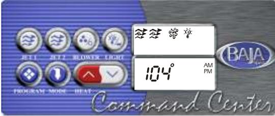
The In-House Control Panel shares the same functions and has the same features as the spaside control panel located within the spa.
