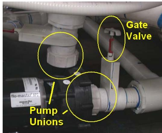
7. Remove the shipping bolts from the base of each pump and rotate the swivel lock, located at the rear of each pump, away from the pump.
