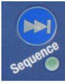
The Sequence button allows you to choose between the six different message sequences. The light glows to indicate the current sequence.
