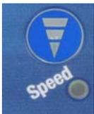
The Speed button changes the amount of time between each step of the massage sequence. *The default time is 5 seconds.* Push the Speed button once to change it to 15 seconds, again to change it to 30 seconds. A third push will return it to 5 seconds. The status light below the Speed button will blink at the current speed.
