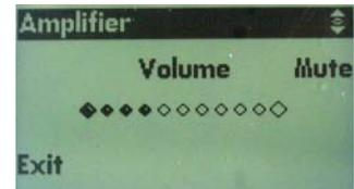
Press Mute to temporarily turn off the amplifier's speakers. Push Mute again to turn the speakers back on.
