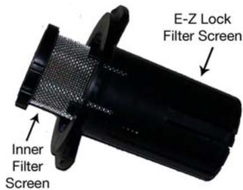
Then remove the Inner Filter Screen and clean both screens with water, using pressure from the **inside** of each screen.
