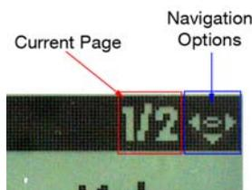
The amplifier and settings menus both contain two pages of options; the page you are currently on is indicated in the top right of the display. On the 5-Key Context Keypad, the up and down buttons scroll between pages 1 and 2 in that particular menu. The center button takes you back to page 1 of the current menu; if you are at page 1, it takes you back to the Temperature menu. If you are adjusting a setting (i.e. bass), the center key takes you back to the menu you accessed that setting from.
