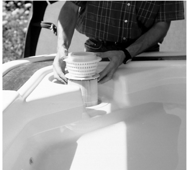
(Figure V) Skimmer, Basket & Filter Location
