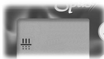
**Pumps have started up for one minute on several occasions and "Filter Cycle" icon is flashing.**
