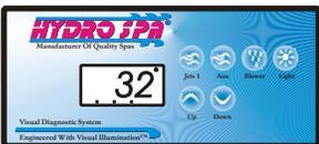
If the display shows a constant 32 degree F or 125 degree F and this is not the actual temperature or the displayed temperature greatly differs from the actual spa water temperature, a problem with the water temperature sensor has occurred. (Contact your spa dealer or manufacturer).
