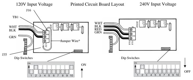
\*Jumper wire attached to rear of power system enclosure
