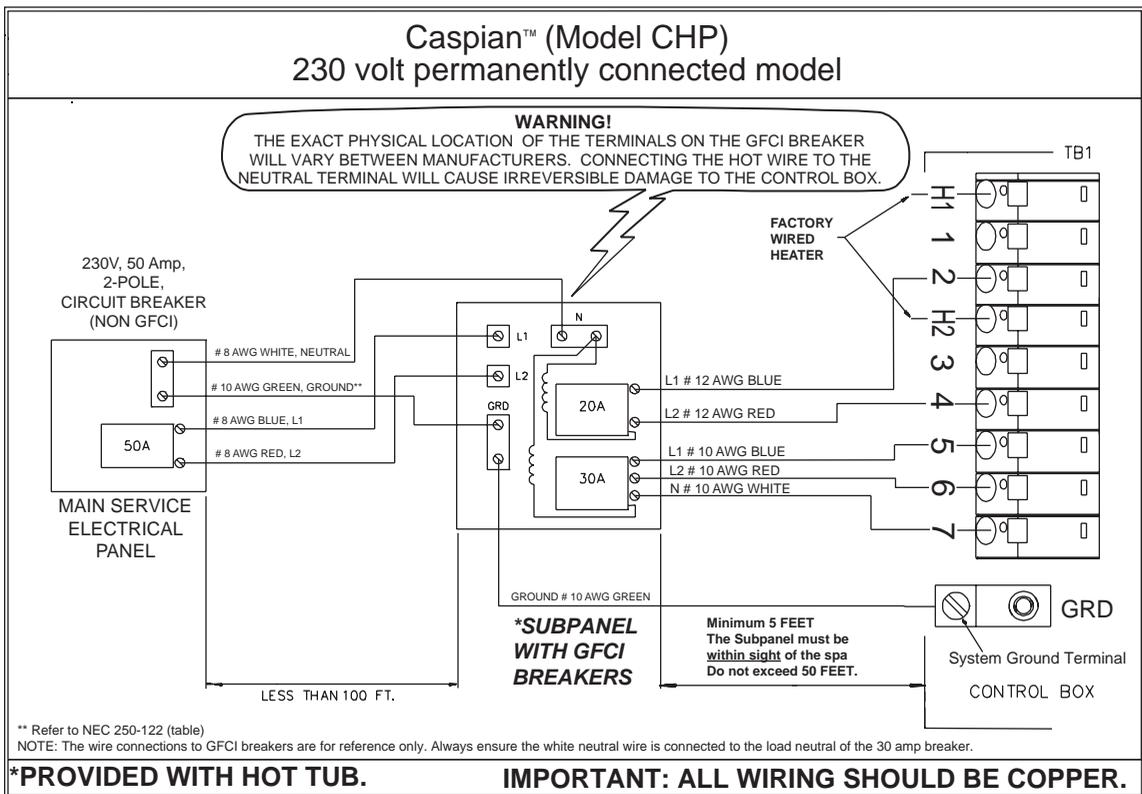
**NOTE:** Long wiring runs may require larger-gauge wire than stated.
