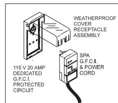
If the GFCI fails to operate in this manner, your spa may have an electrical malfunction, and you may be risking electrical shock. Turn off all circuits and do not use the spa until the problem has been corrected by an authorized service agent.
