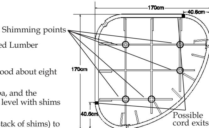
6. Use the carpenter's level to recheck the level of the spa.
