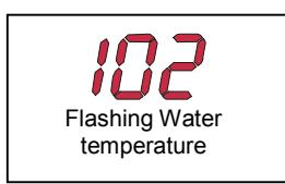
If the temperature flashes on the display, the power has been disconnected from the spa and the flashing display indicates the default settings were restored when power was connected.
