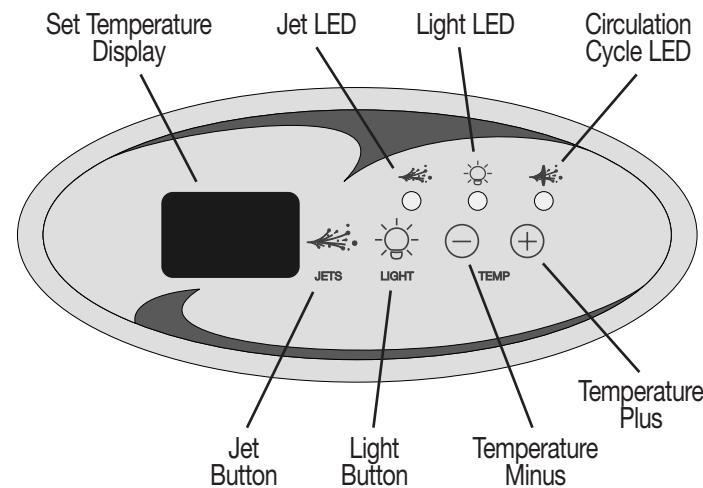
C. TEMPERATURE CONTROLS: The set temperature range is from 50°F to 104°F (10°C to 40°C).
