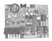
These boards use the same mounting footprint as older circuit boards to simplify replacement. Refer to the table below for compatibility information and complete jumper selection details. <u>To ensure optimum performance, always remember to verify all circuit board jumper settings and spa functions before leaving the work site.</u>
